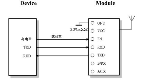
Notes: When join TTL interface, Please don't join in 6PIN and 7PIN
