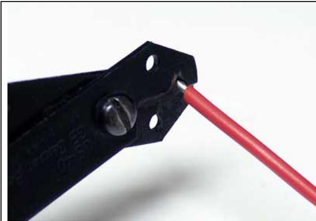
**Step 1:** Strip the wire which you are using approximately 1/4". The wires may be 12 gauge to 30 gauge. Use thicker wire for high current applications.
