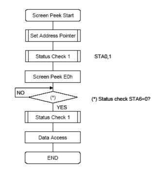
Note: This command is available when hardware column number and software column number are the same. Hardware column number is related to MD2 and MD3 setting. Software column number is related to Set Text Area and Set Graphic Area command.
