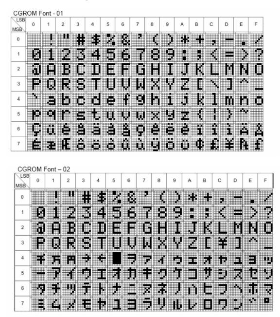
The RA6963 has two part number - RA6963L2NA and RA6963L2NB. The RA6963L2NA is compatible to T6963C(code 0101) and the default font is Figure 6-13 as above. The RA6963L2NB is compatible to T6963C(code 0201) and the default font is Figure 6-14 as above. Although RA6963 provide a extra internal command for MCU to select both font of above, but you do not need to change the software to select the font that if you chose the right part number.
