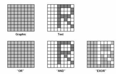
Note: Attribute functions can only be applied to text display, since the attribute data is placed in the graphic RAM area.
